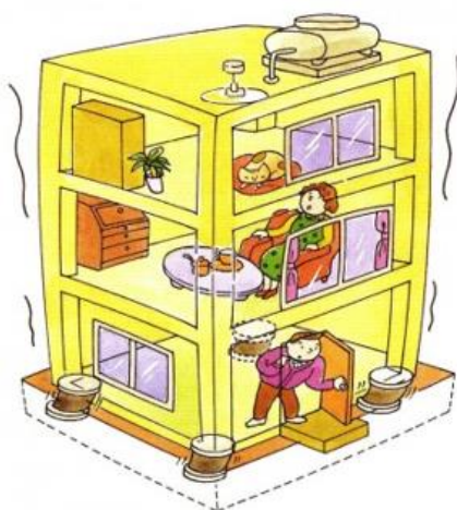
Building with Seismic Isolation
