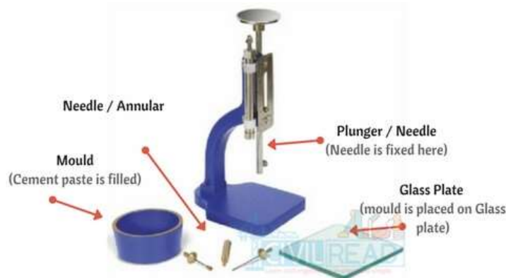
VICAT Apparatus with details
