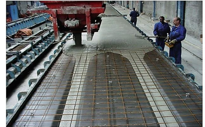
Figure 5.58 Self-compacting concrete grade C50/60 is often used for wet-casting double-tee slabs (courtesy of EFNARC).
