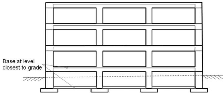
Figure A1.2 Building with Basement where the Base is at the Level Closest to Grade Elevation
