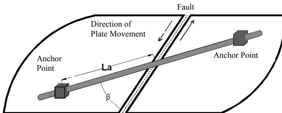
Figure 13.2 Pipeline Crossing a Strike Slip Fault
