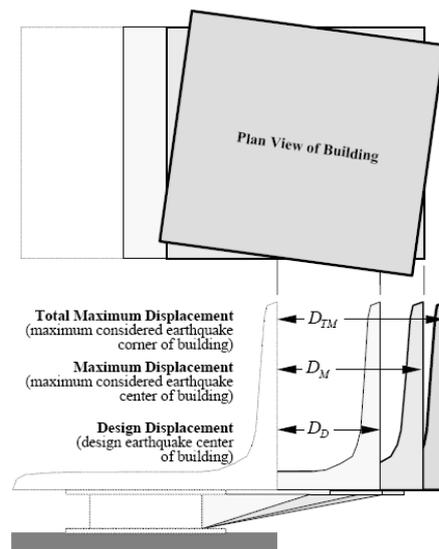
Figure 9.1 Displacement Definition
