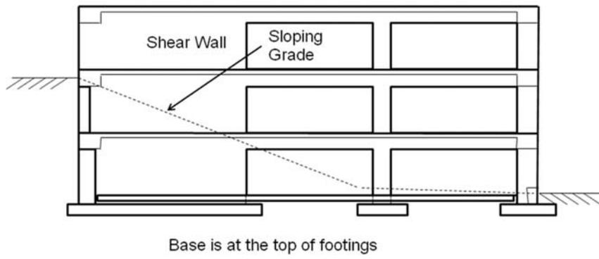
Figure A1.6 Building with Shear Walls which also Resis Soil Lateral Pressure
