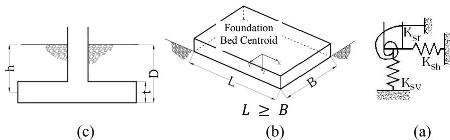
Figure 5.1 Parameters for Equations. 5.10 & 5.11
