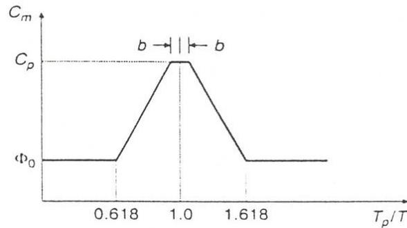
Figure 8.2 Variation of Modified Amplification Factor with Respect to Different Fundamental Periods
