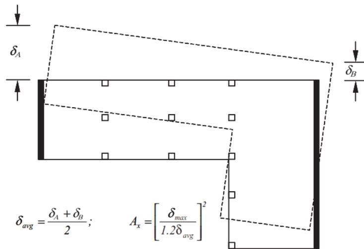
Figure 4.5 Average Lateral Displacement at Each Level
