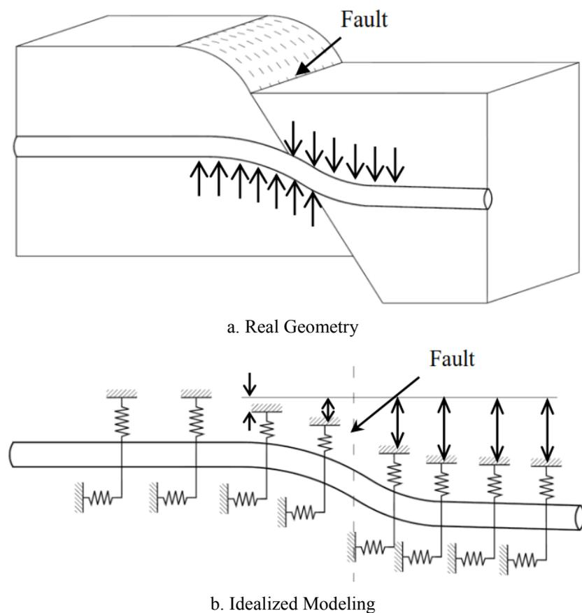
Figure 13.4 Modeling of Pipeline for Fault Displacement
