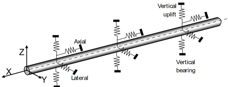
Figure 13.7 Modeling Soil-Pipe Interaction with Inelastic Springs
