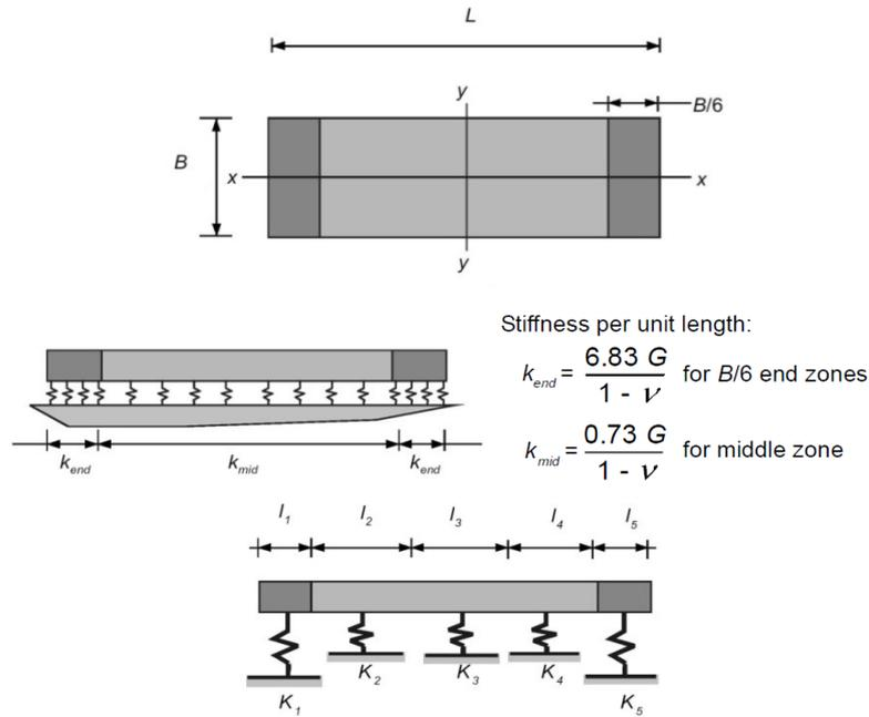
Each spring stiffness:  $K_{j,emb} = l_i k \beta_z$  where  $\beta_z$  is determined from Equation 5.11
