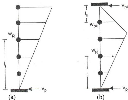
Figure 8.1 Hypothetical 1<sup>st</sup> Mode Shape for Non-Structural Components by Connections in One or Two Points
