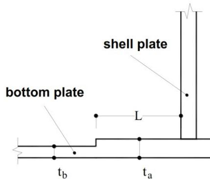
Figure 12.2 Dimensions of Shell Annulus and Bottom Plates
