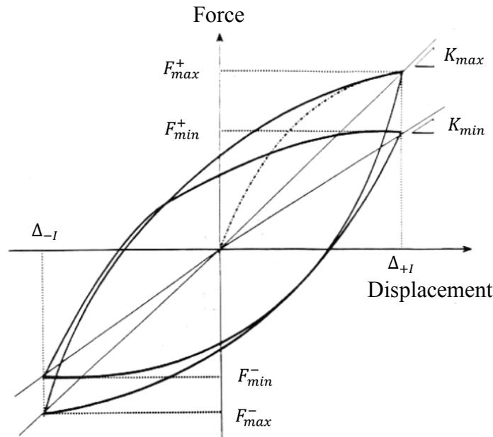
Figure 9.3 Stiffness Effects on Cyclic Behavior of Isolators
