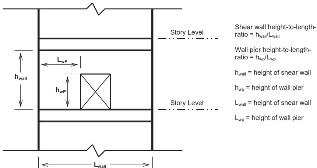
Figure 4.2 Shear Wall and Wall Pier Height-to-Length Ratio Determination
