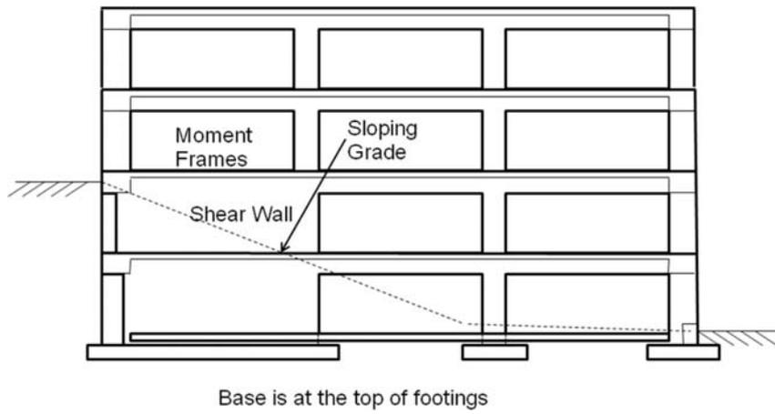
Figure A1.7 Building with Retaining Wall Connected to the Structural System
