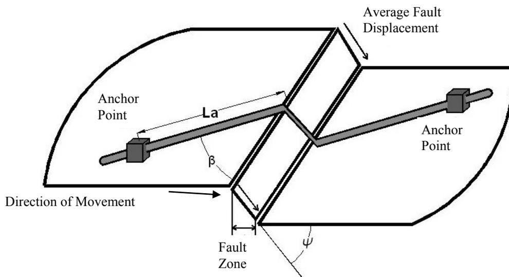
Figure 13.3 Pipeline Crossing a Normal Slip Fault
