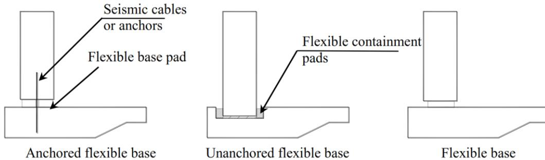
Figure 12.4 Flexible Base Connections
