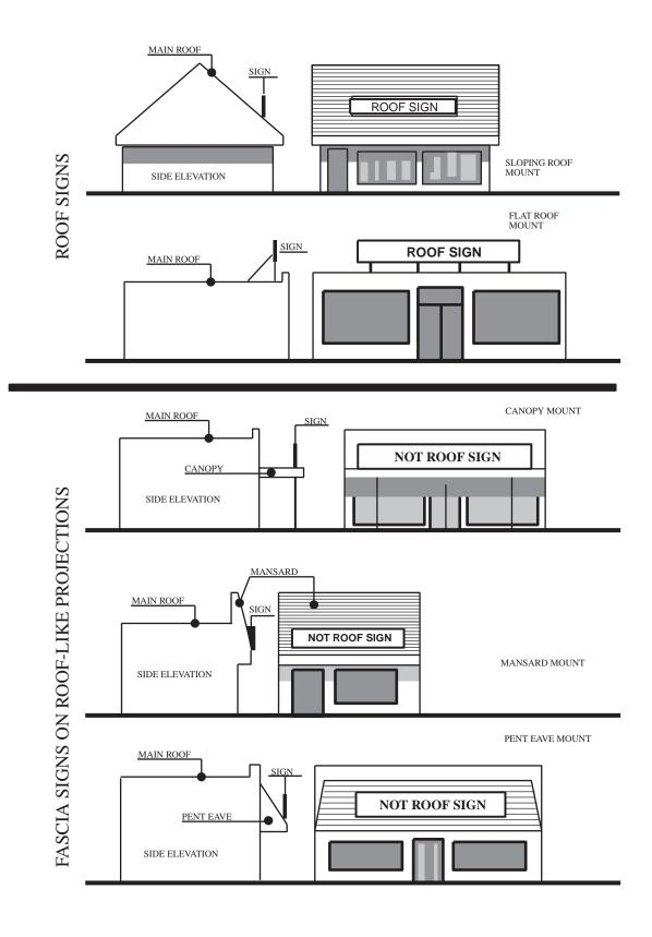
FIGURE 1003.1(2) COMPARISON—ROOF AND WALL OR FASCIA SIGNS
