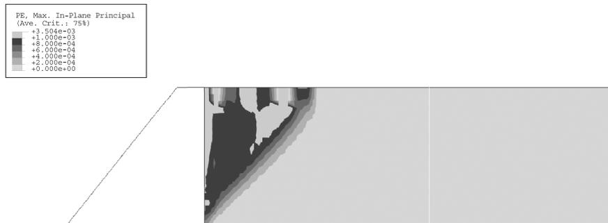
FIGURE 7.30 Distribution of plastic strains in the backfill at active failure.
