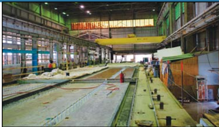
Deck panels are fabricated in this large precast plant in New Jersey.
