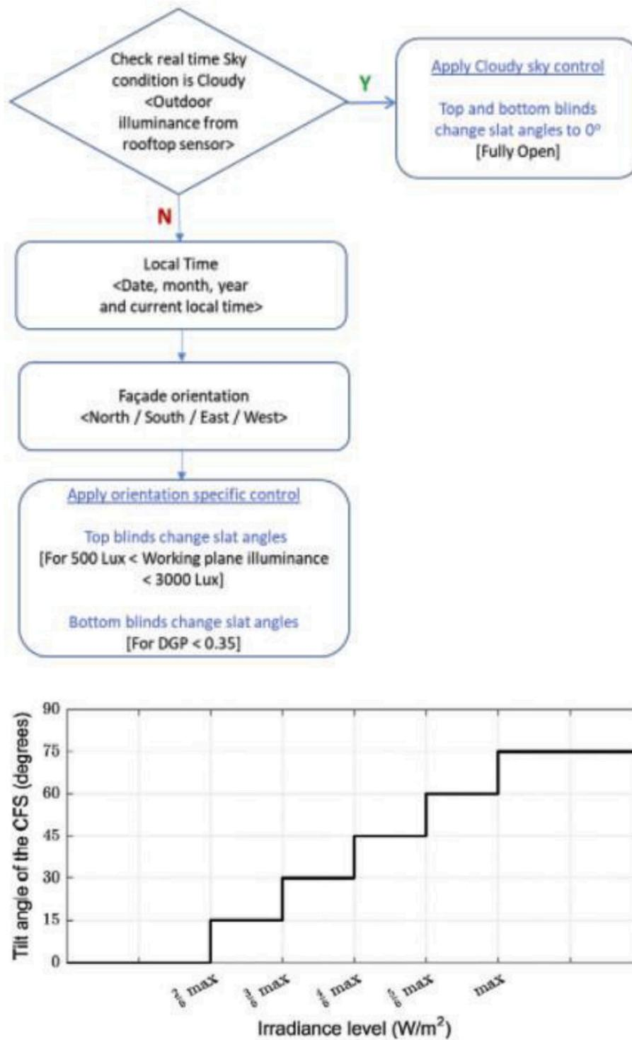
Fig. 4. (Top) Adapted control algorithm in Ref. [72], (Bottom) Slat angle control strategy [73].
