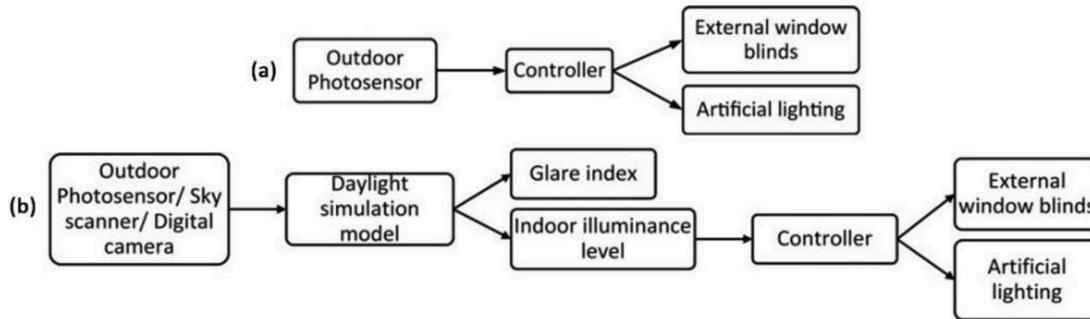
Fig. 3. Conventional (a) and Model-based (b) open-loop algorithms [10].
