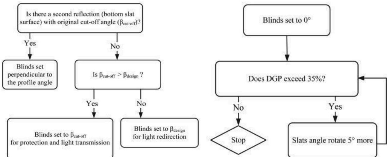
Fig. 6. Daylight redirection (left) and glare control (right) control algorithms adopted in Ref. [66].
