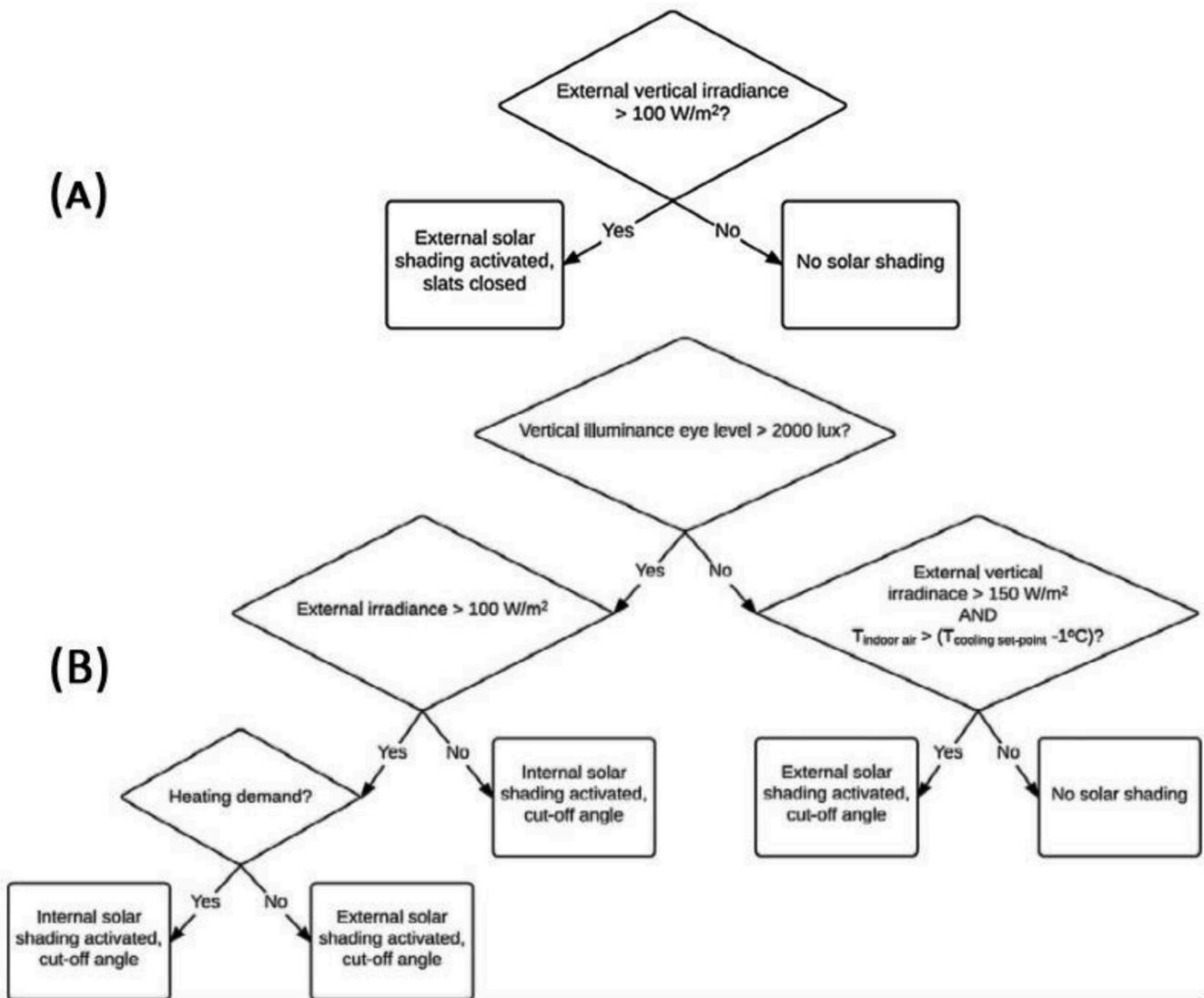
Fig. 5. Typical simple (A) and detailed (B) control algorithms adopted in Ref. [75].
