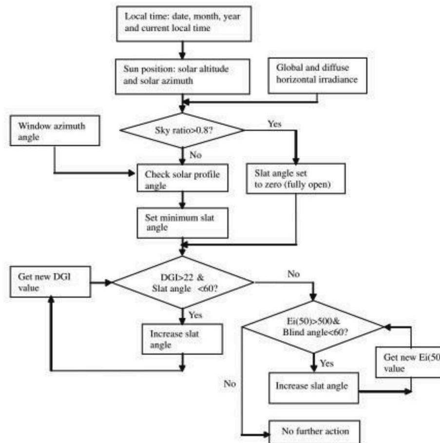
Fig. 13. A closed-loop control to control glare [64].
