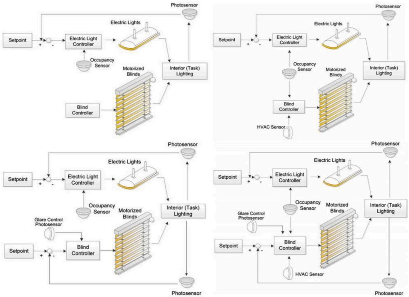
Fig. 11. Examples of independent control loops [68].
