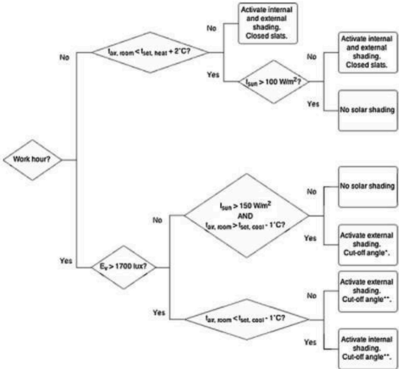
Fig. 7. Open-loop control based on occupancy activity [67].
