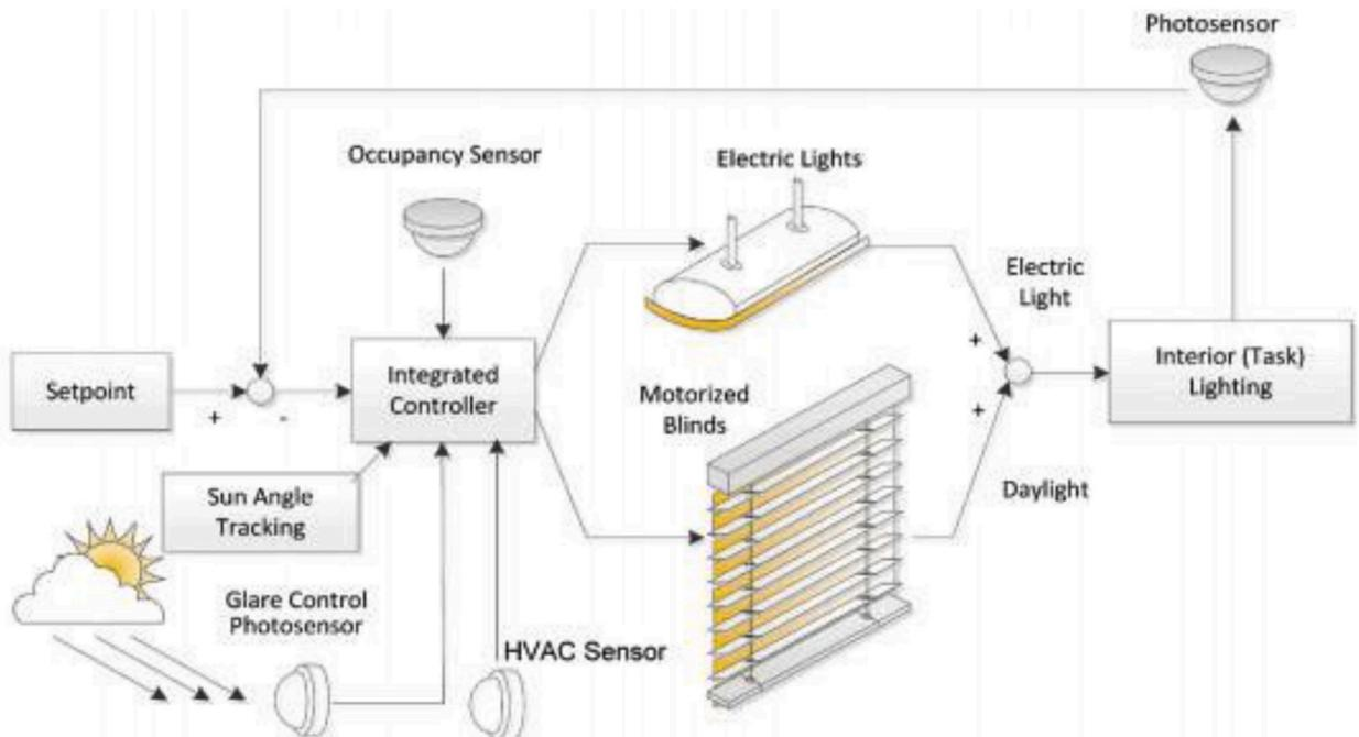
Fig. 12. Example of an integrated control loop [68].
