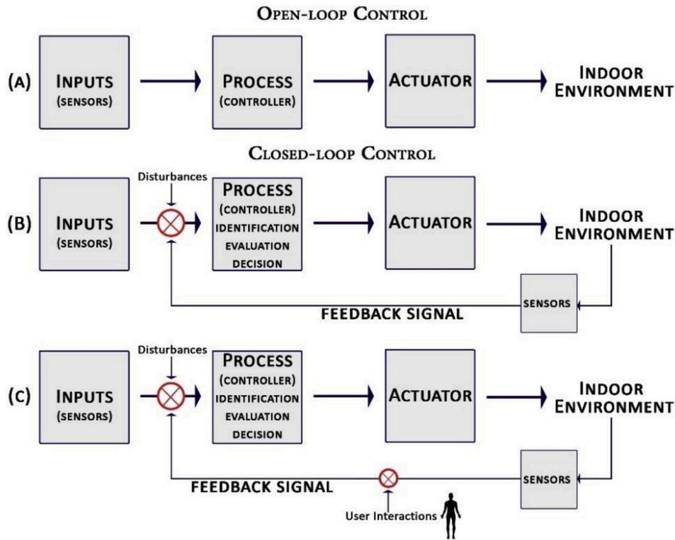
Fig. 2. Open-loop and Closed-loop control algorithms.
