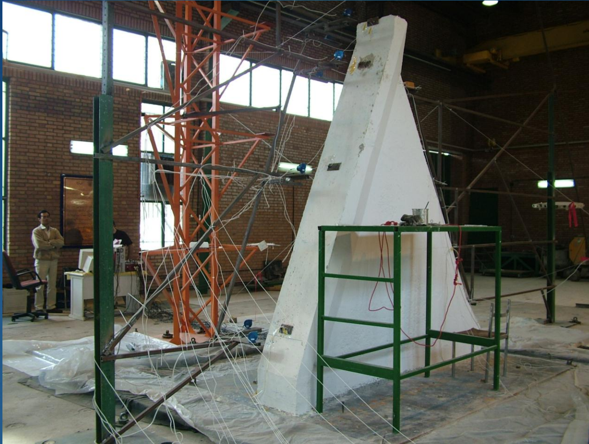
Concrete Dam Model tested under real Earthquake record
