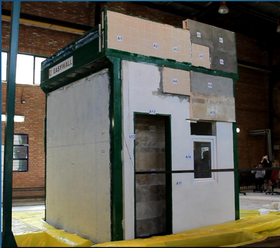
EasyWall panels tested under Zarand Earthquake record
