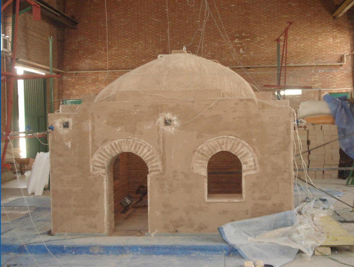
Adobe Dome-Roof building tested under real Earthquake record
