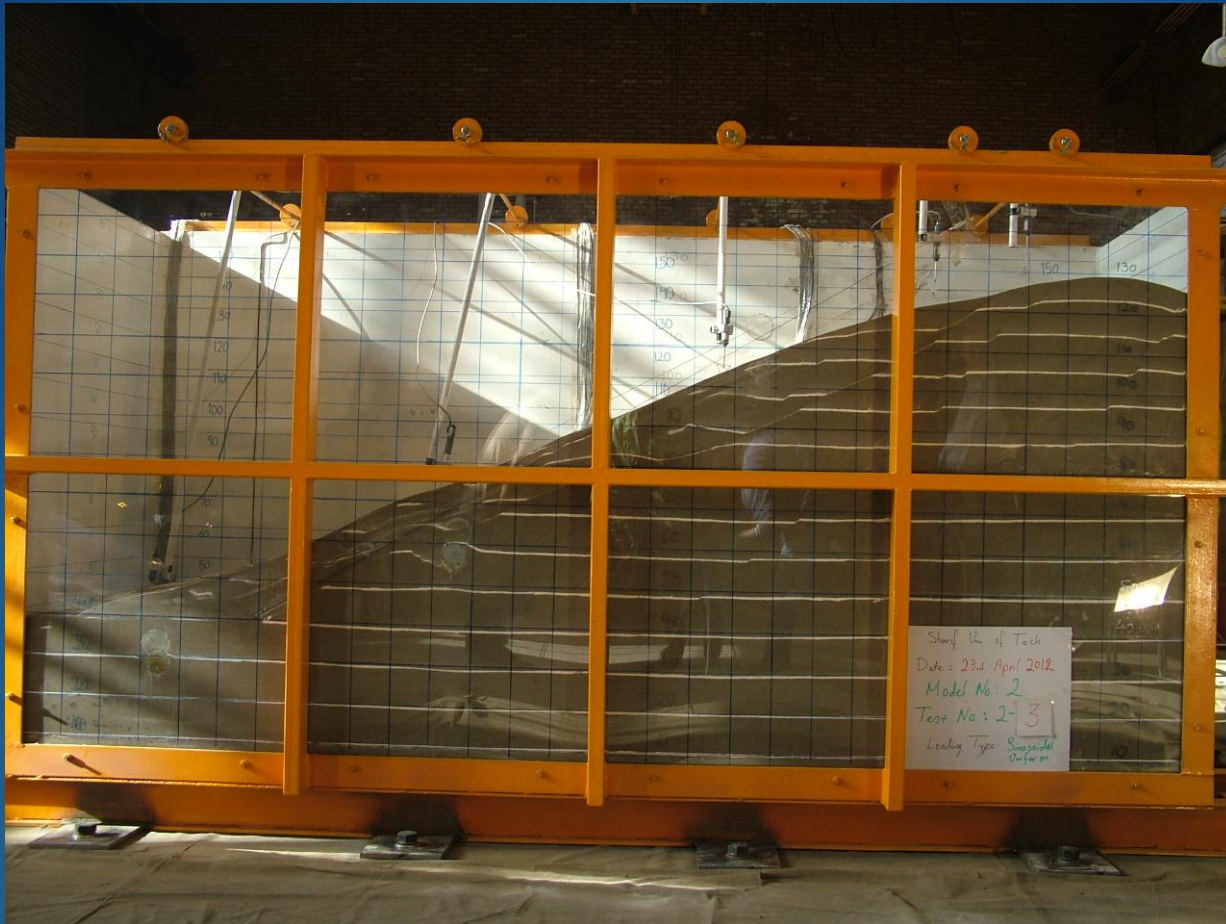
Pipeline model tested under Harmonic excitations
