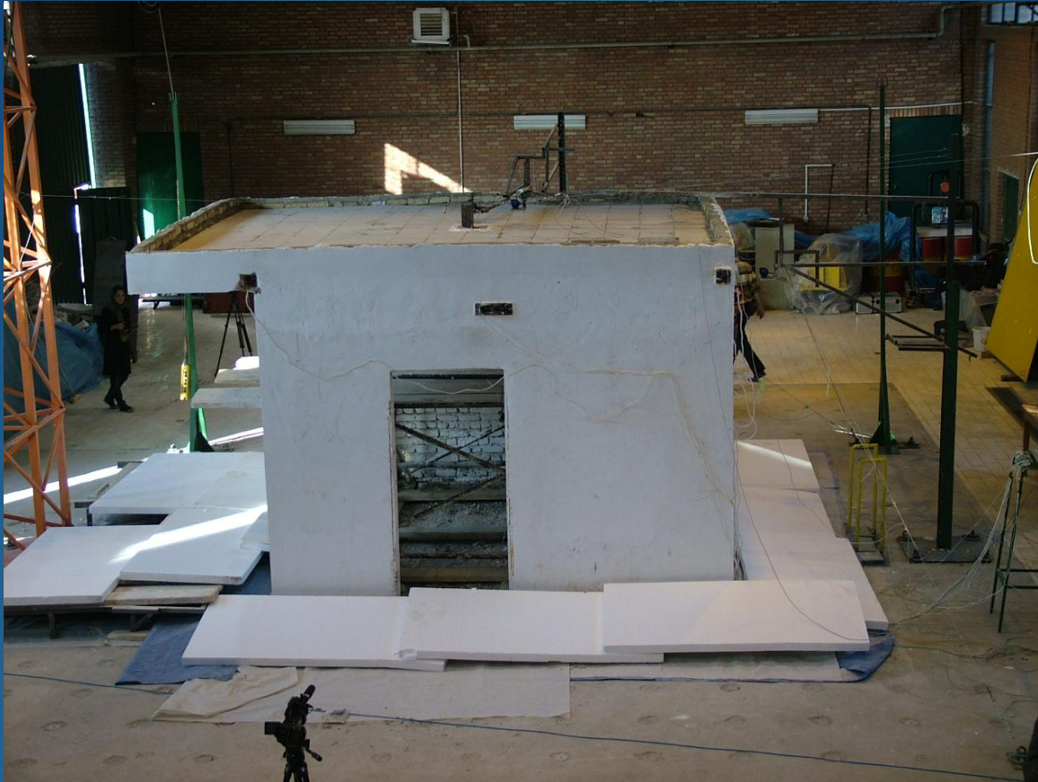
Brick-Masonry building tested under real Earthquake record
