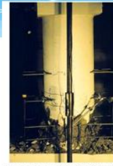
Loss of Axial-Load Capacity (Column P2)
