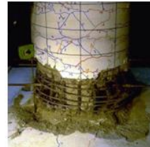
Loss of Axial-Load Capacity (Column P2)
