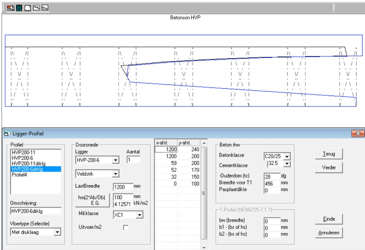
RSLProf.exe is a program to access the library with pre-defined slabs, plate systems with multiple reinforcement patterns. An slab can be implemented by added cast as a topping or adjacent. The properties which are relevant for the calculation are being abstracted, such as the location of the channels and positions of the reinforcement. The section coordinates are being compressed on the y-axis.
