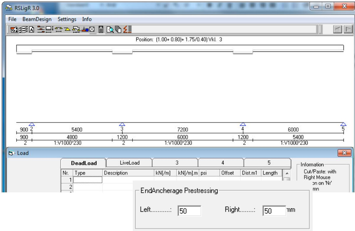
Almost all beam design software is developed being design software, RSLigR is characterized to be a production tool. The application focuses on floors but may also be used to design beams, precast or in-situ. The user is assisted by defaults that may be changed. The menu structure is flat and scarcely needs to be addressed since apart from the buttons a click in the graphics window leads to the relevant section.
