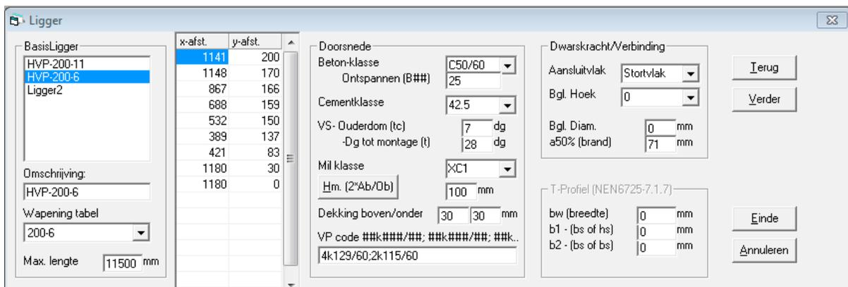
Reinforcement patterns may consist of four layers that need to be introduced bottom-up in order and distance. Max. elementlength may be connected to a reinforcement pattern or each element. If both were introduced the length of the rebarring will have first priority.
