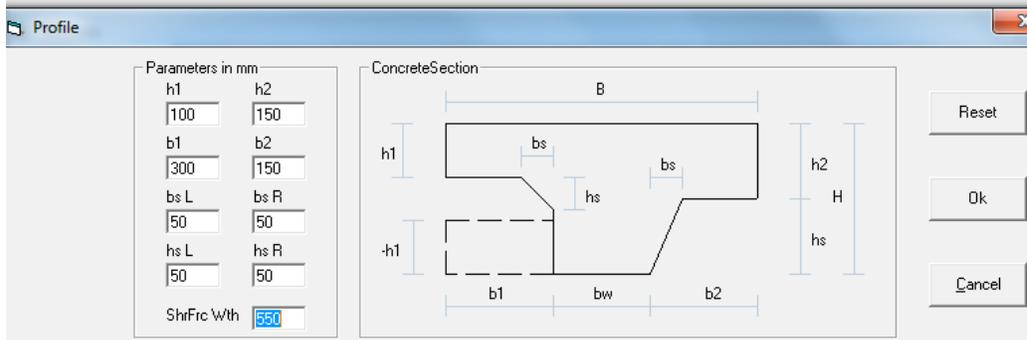
Costs calculation data for wide-slab floors are accessible at each girder and each component totals and averages. Traditional reinforcement in kg/m<sup>2</sup> and for patterns of tension as surface amount.
