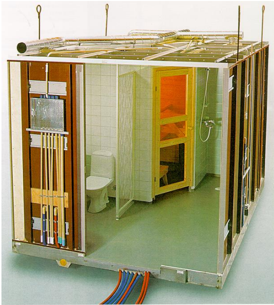
Fig. 1.2.18 Box module cells are often supplied with electric conduit and boxes, furniture, window and door embedments, and mechanical and plumbing chases cast in, reducing costly field work.
