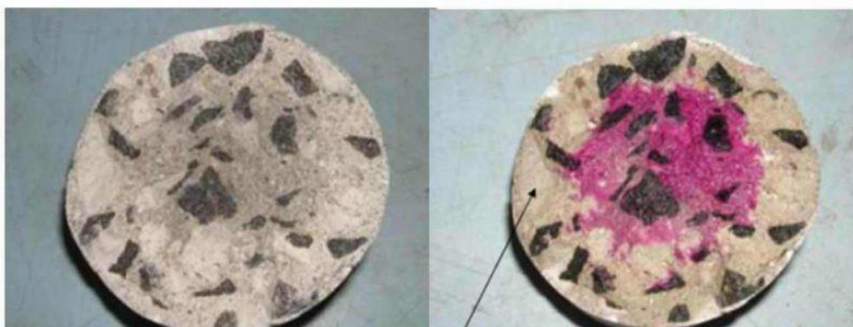
Concrete Exposed To CO_2
