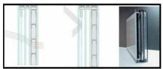
Figure 2. Window section with salt hydrates insulation, summer and winter (Ritter, 2007)
