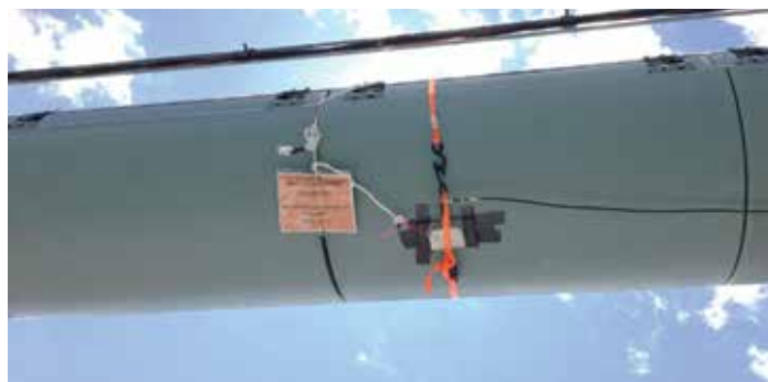
Figure 8 and 9. Tri-axial accelerometers attached to the bridge. Courtesy of Thornton Tomasetti Weidlinger.
