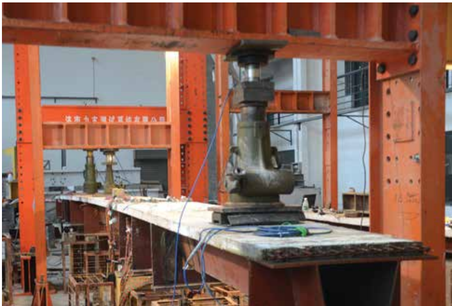
Figure 3. Set-up of the static load test.
