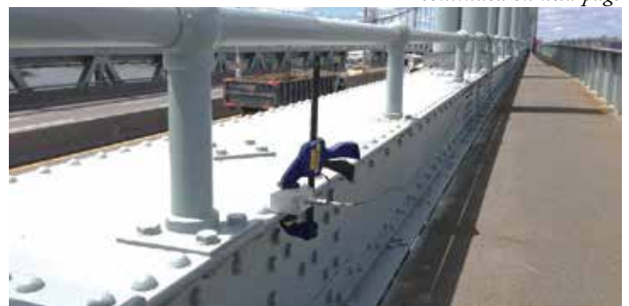
Figure 8 and 9. Tri-axial accelerometers attached to the bridge. Courtesy of Thornton Tomasetti Weidlinger.
