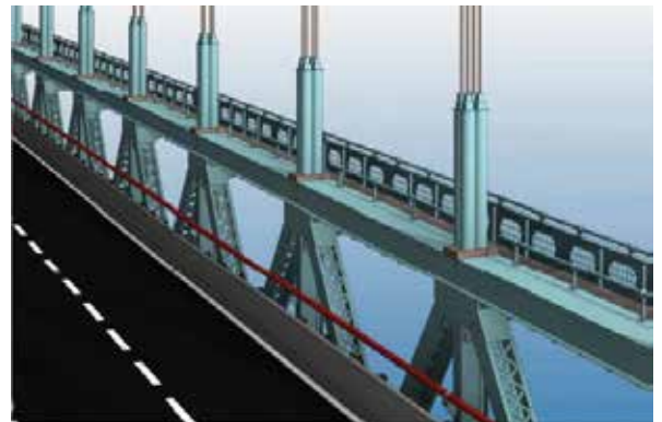
Figure 4. Perforations in sidewalk fascia girder.
