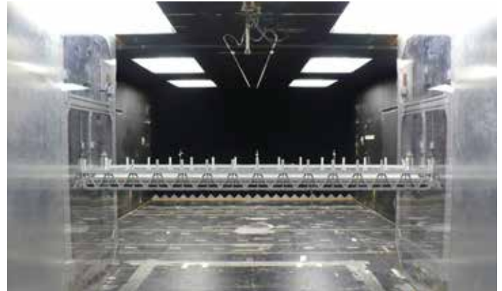
Figure 2. Wind section model of the RFK Bridge. Courtesy of Boundary Layer Wind Tunnel Laboratory.
