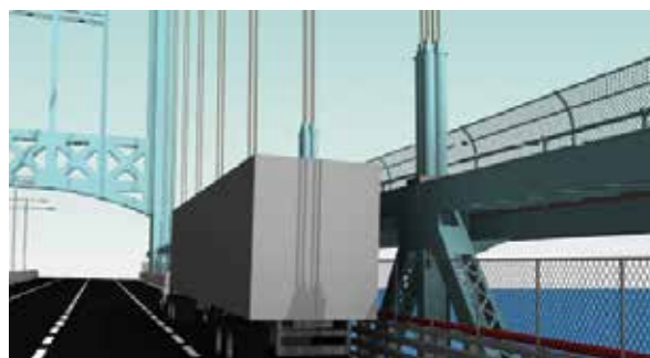
Figure 10. Shielding effects of bridge stiffening truss.
