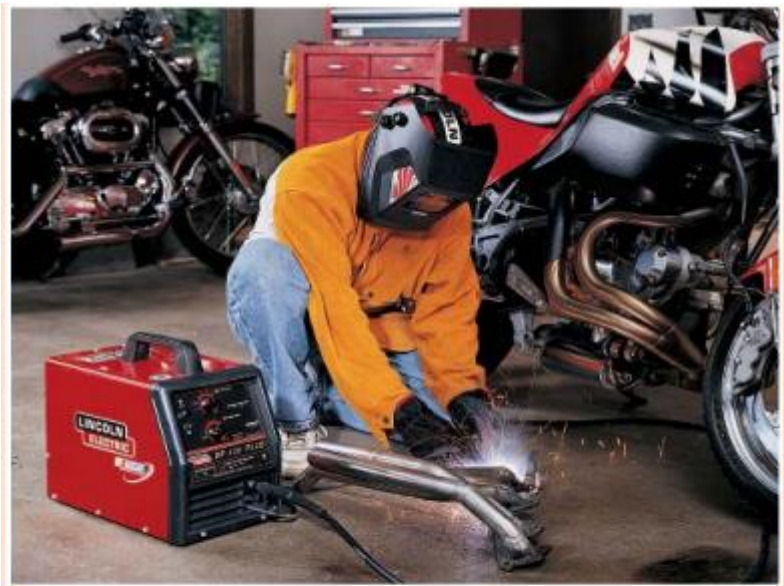
Figure 3: Small, portable 120 volt wire feeder/power source combinations may look lightweight, but when produced by a reputable welding manufacturer, they can be ideally suited for welding on gage materials—even for structural applications.
