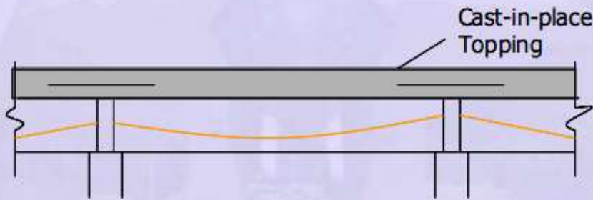
c) Composite construction with continuity reinforcement
