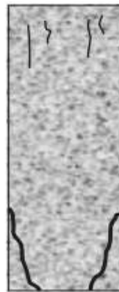
Cracks due to increased column load
