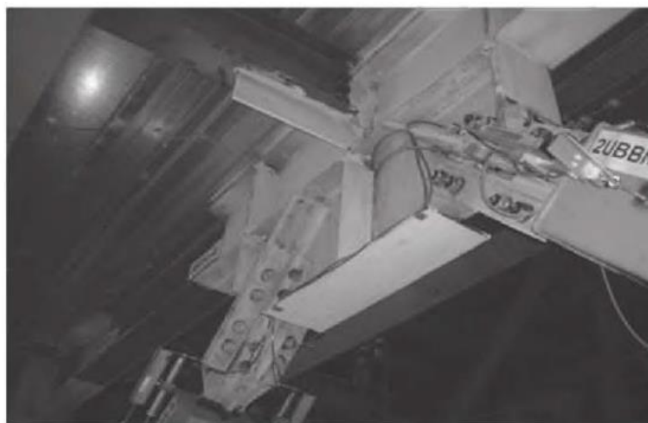
(b) Edge-stiffened gusset connection
